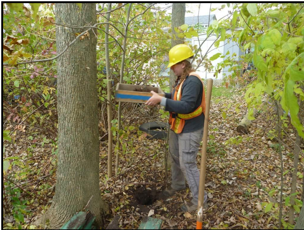
Image 12: View of Crewmember Screening Soil through 6 mm Mesh (Photo Taken on October 15, 2012; Facing West)
